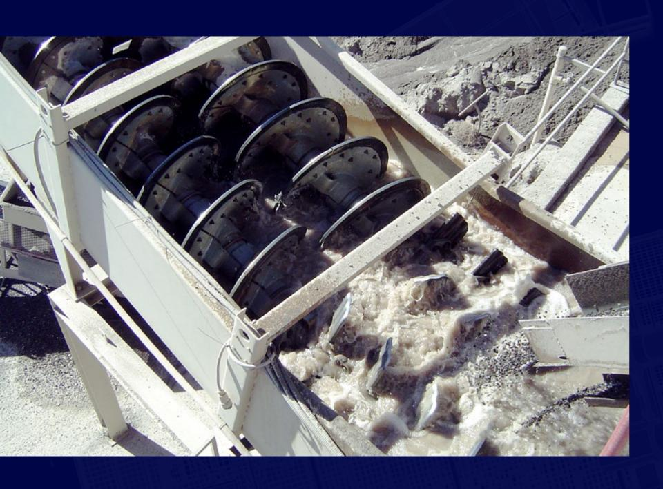
Coarse Material Washers are used for Light Scrubbing applications.
