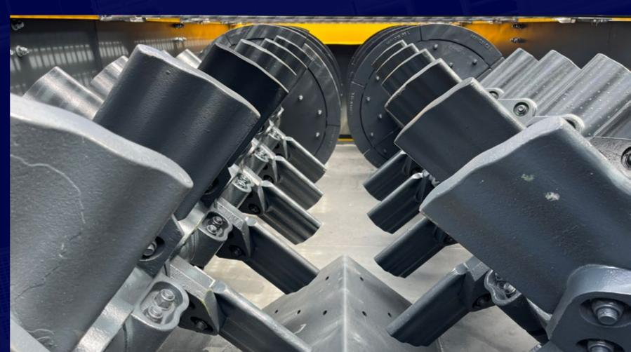
Paddles also provide jigging action to float up sticks, roots, and lightweight matter to be flushed out over the feed end of the tub by the rising current.
